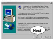
When asked to install or remove the audio driver, please select "Install" and press "Next" button to continue.
