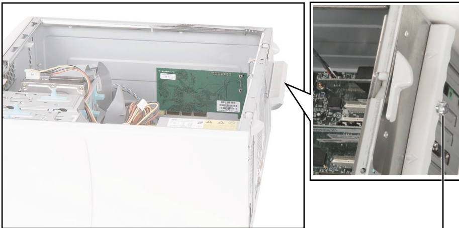
Card retention cover thumb-screw
