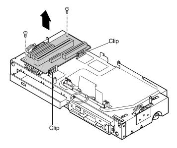
**5** Install the new connector board:
