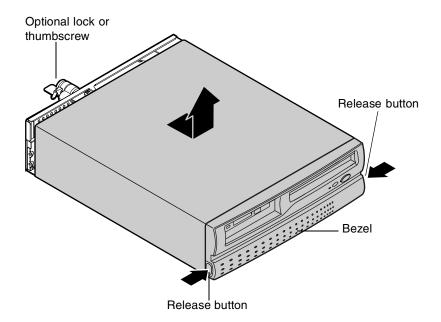
**4** Lift the cover up and off the chassis.
