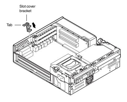
**5** Locate an available slot and pull out the slot cover.
