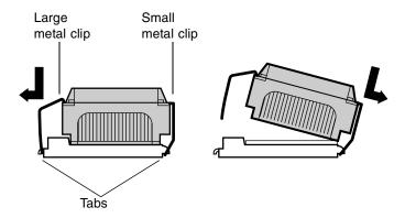
**c** Lift the heat sink at an angle and unhook the small metal clip. Lift the heat sink off the processor.
