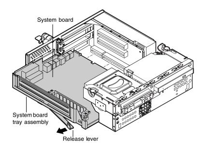
Grasp the edge of the tray and carefully slide the tray out of the chassis.
