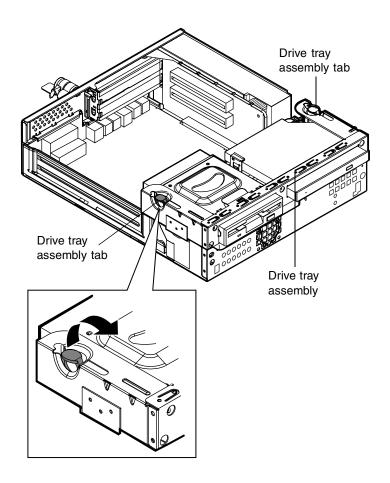
**b** Tilt the drive tray slightly forward while lifting it up and off the chassis.
