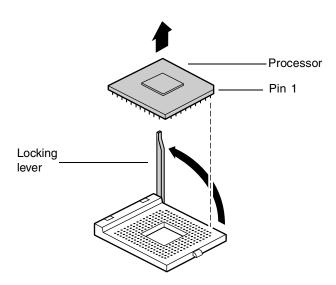
**b** Lift the old processor straight up and out of the socket.
