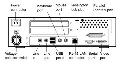
**Line-in and line-out audio jacks** connect audio devices such as speakers and a microphone.
