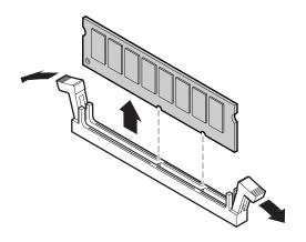
**5** Insert the DIMM into the socket and align the two bottom notches i the DIMM with the two notches in the DIMM socket.
