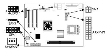
Connect power supply to the **ATXPW1** connector on the mainboard. **CN1** is the CPU Vcore power connector. If there is a cooling fan in the system chassis, connect the cooling fan cable to the **SYSFAN1** fan power connector on the mainboard. Connect the PC speaker cable to the **SPK1** header on the mainboard.
