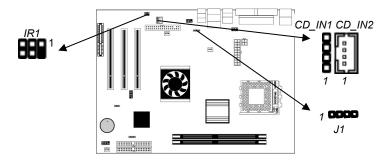
On the mainboard, locate the two 4-pin connectors **CD\_IN1** and **CD\_IN2**. There are two kinds of connector because different brands of CD-ROM drive have different kinds of audio cable connectors. Connect the cable to the appropriate connector.
