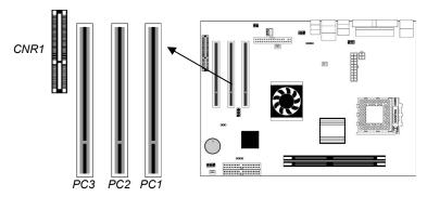
Follow the steps below to install a PCI/CNR expansion card.
