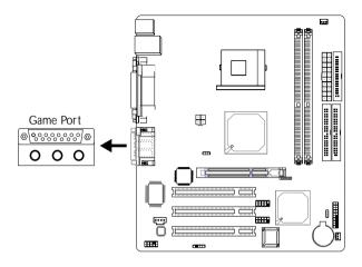
The Game/MIDI port is identical to that of a standard PC game adapter or game I/O port. Connect an analog joystick to the 15-pin D-sub connector (Gold) at location CN9 of the system board. This port works well with any application that is compatible with the standard PC joystick.
