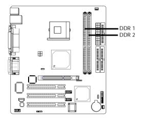
The system board is equipped with two 184-pin DDR SDRAM DIMM (Dual In-line Memory Module) sockets that support 2.5V DDR SDRAM DIMM. Double Data Rate SDRAM (DDR SDRAM) is a type of SDRAM that doubles the data rate through reading and writing at both the rising and falling edge of each clock. This effectively doubles the speed of operation therefore doubling the speed of data transfer.
