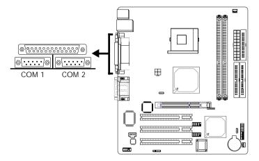
The system board is equipped with onboard serial ports (COM 1: CN6 and COM 2: CN5) - both in Teal/Turquoise color.
