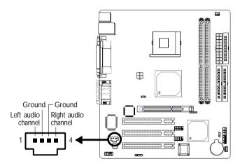
The CD-in connector (J3) is used to receive audio from a CD-ROM drive, TV tuner or MPEG card.
