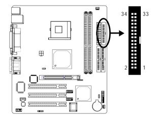
The system board is equipped with a shrouded floppy disk drive connector for connecting a standard floppy disk drive. To prevent improper floppy cable installation, the shrouded floppy disk header has a keying mechanism. The 34-pin connector on the floppy cable can be placed into the header only if pin 1 of the connector is aligned with pin 1 of the header.
