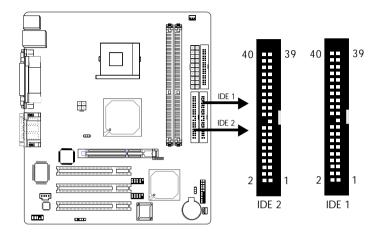
The system board is equipped with two shrouded PCI IDE headers that will interface four Enhanced IDE (Integrated Drive Electronics) disk drives. To prevent improper IDE cable installation, each shrouded PCI IDE header has a keying mechanism. The 40pin connector on the IDE cable can be placed into the header only if pin 1 of the connector is aligned with pin 1 of the header.
