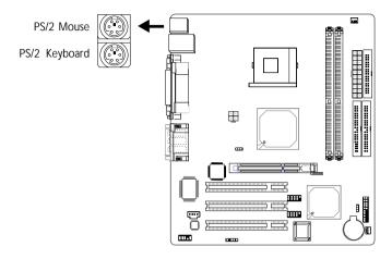
The system board is equipped with an onboard PS/2 mouse (Green) and PS/2 keyboard (Purple) ports - both at location CN1 of the system board. The PS/2 mouse port uses IRQ12. If a mouse is not connected to this port, the system will reserve IRQ12 for other expansion cards.
