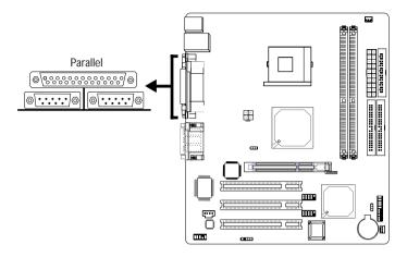
The system board has a standard parallel port (Burgundy) at location CN8 of the system board for interfacing your PC to a parallel printer. It supports SPP, ECP and EPP modes.
