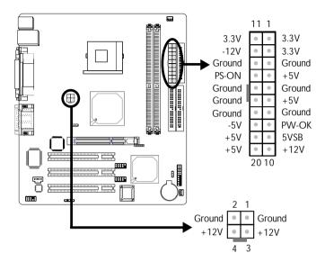
Use a power supply that complies with the ATX12V Power Supply Design Guide Version 1.1. An ATX12V power supply has a standard 20-pin ATX main power connector and a 4-pin +12V power connector that must be inserted onto CN11 and CN10 connectors respectively.
