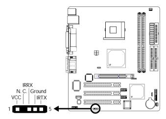
Connect your IrDA cable to connector J5 on the system board.
