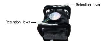
4. Move the retention levers to their opposite directions then push them down. This will secure the fan / heat sink and retention mechanism assembly to the retention module base.
