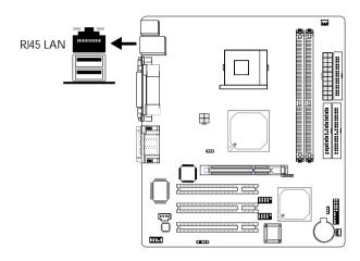
The system board is equipped with an onboard RJ45 fastethernet LAN port at location CN7 of the system board. It allows the system board to connect to a local area network by means of a network hub.
