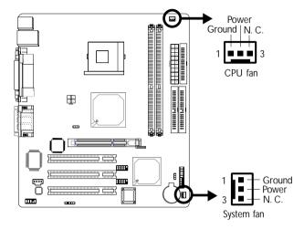
Connect the CPU fan's cable connector to the CPU fan connector (J8) on the system board. The system fan (J12) connector is used to connect an additional cooling fan. These cooling fans will provide adequate airflow throughout the chassis to prevent overheating the CPU and system board components.
