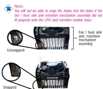
3. The retention levers at this time remains unlocked as shown in the illustration below.
