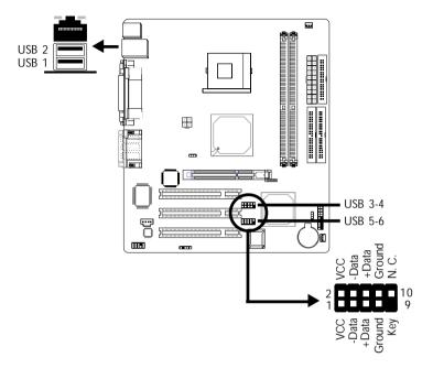
Two onboard USB ports (Black) are at location CN7 of the system board.
