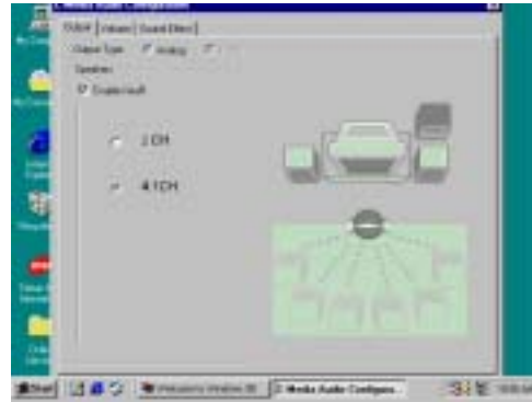
10. When Enabled XeaR, you can plug earphone in Speak-Out connector as a Rear speaker, and 2-channel speaker plug in Line-In as Front Speaker to get 4-channel effect
