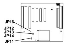
JP11, J12, J13, J14, JP16 - Power Selection for the CPU Core Voltage, Bus Section and Bus Voltage
