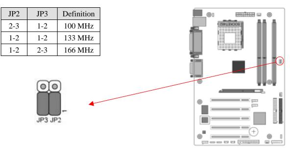
This cap setups up the CPU Ext. Clock Frequency. This function allows you to set the CPU's FSB. The default setting is at pin [1-2], and your CPU's FSB will be automatically detected.
