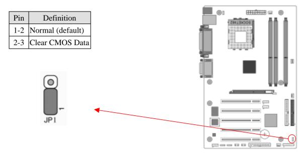
There is a CMOS RAM on board that has a power supply from external battery to keep the data and system configuration. To clear the contents of the CMOS, please follow the steps below.
