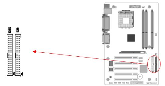
The motherboard has a 32-bit Enhanced PCI IDE and Ultra ATA66/100/133 controller that provides PIO mode 0~4, Bus Master, and Ultra ATA66/100/133 function. This connector is used for connecting 40 pins of ATAPI devices.
