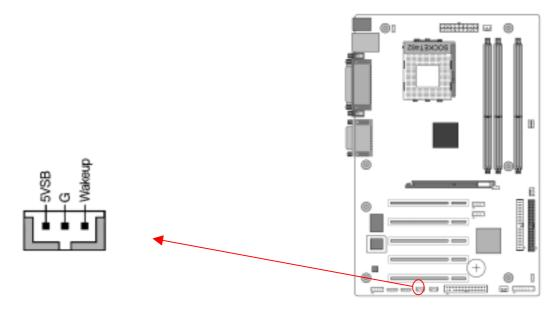
Enable the Wake Up On LAN selection in BIOS's Power Management Menu to use this function. The capability to remotely manage PCs on a network is a significant factor in reducing administrative and ownership costs. Magic Packet technology is designed to give WOL capability to LAN controller. This header is used to connect an add-in NIC (Network Interface Card) that gives WOL function to the motherboard.
