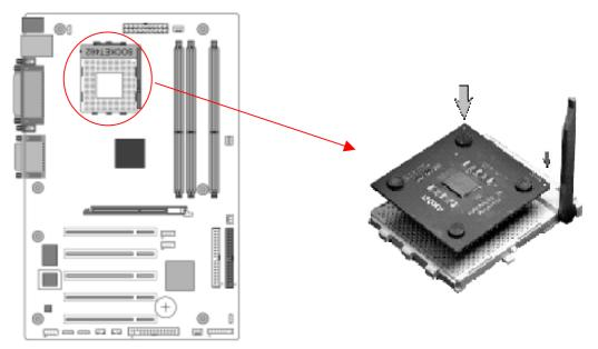
*Note*: In order to boot up with a newly installed CPU, AC Power must be switched off before installation.
