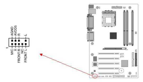
This connector gives you the option of a front-panel audio jack cable ext. to be plugged into a special custom-designed system case.
