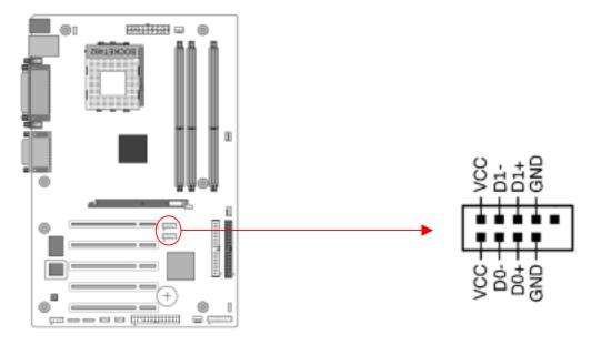
CN23/CN23A (Front USB Connector for USB 2/3 and 4/5)
