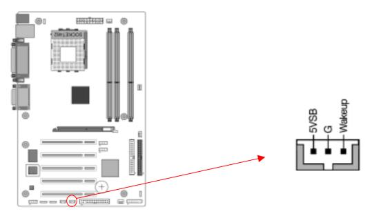
Enable the Wake Up On Modem selection in BIOS's Power Management Menu to activate this function. This header is used to connect an add-in modem card, which gives WOM capability to the motherboard.
