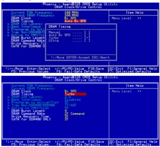
4. Adjust the setting of DRAM Timing to [Turbo]
