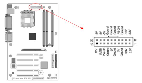
**PW1 (ATX Power Supply Connector)**
