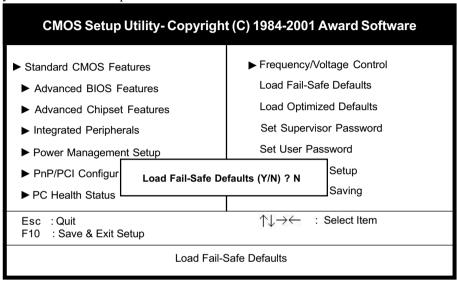
Figure 3-10 Load Fail-Safe Defaults Screen
