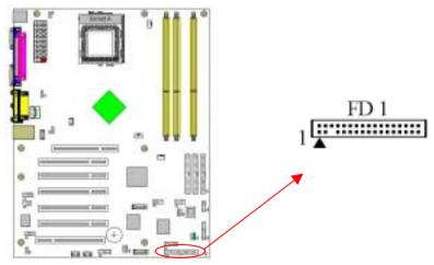
This connector is used to connect 34 pins of Floppy.
