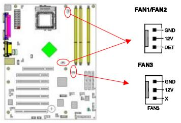
The board's management extension hardware is able to detect the CPU and system fan speed in rpm (revolutions per minute). The wiring and plug may vary depending on the manufacturer. On standard fans, the red is positive (+12V), the black is ground, and the yellow wire is the rotation signal.
