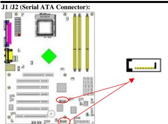
This can connect to new IDE device, it support ATA 150MB/sec. Notes: Setup problem, please refer to Appendix Serial ATA/IDE RAID. JP1 (Clear CMOS Data):
