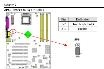
A USB keyboard hot key or a USB mouse click can turn on this board. You must also set this jumper's cap to pins 2-3 to use this function.
