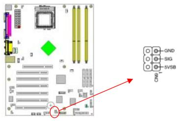
This connector provides a buzzer sound when an attempt to open the chassis occurs.
