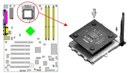
*Notes:* In order to boot up with a newly installed CPU, **AC Power must be switched off** *before installation.*
