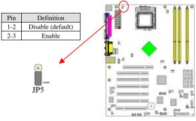
This board can be turned on by the PS / 2 keyboard (hot key). To use this function, select a hot key of your choice at the Hot Key Power ON option under Wake Up Events in the BIOS's Power On Management screen. You must also set this jumper's cap to pins [2-3] to use this function.
