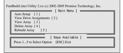
2. Press [1] to display the Auto Setup Menu below. This is the fastest and easiest method to creating your first array.
