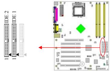
This connector is used for connecting 40 pins of ATAPI devices. IDE 1 only connects two IDE devices. (**Primary** Master/Slave) IDE 2 only connects two IDE devices. (**Secondary** Master/Slave) **IDE 3 (IDE RAID Connector)**
