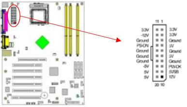
The power cord leading from the system's power supply to the external power source must be the very last part connected when assembling a system. The ATX power supply provides a single 20-pin connector interface, which incorporates standard +/-5V, +/-12V, optional 3.3V and Soft-power signals. The Soft-power signal, a 5V trickle supply is continuously supplied when AC power is available. When the system is in the Soft-Off mode, this trickle supply maintains the system in it's minimum power state.
