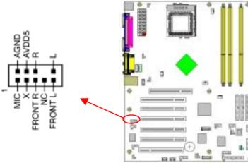
This connector give you the option of a front panel audio jack cable ext. to be plug into a special custom designed system case.
