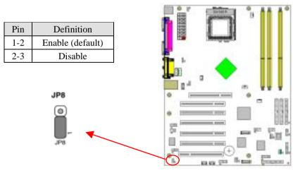
This function allows you to enable or disable the on board audio. You must set the jumper cap to pins **1-2** to **enable** or set pins **2-3** to **disable** this function.
