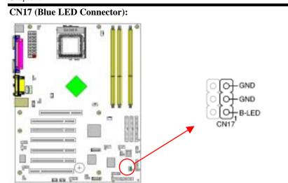
These features work entirely the same as the power indicator LED, both shows the system's power status. The only difference is that this one is blue while the other is red LED.
