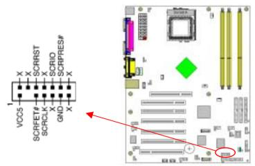
This connector must be connected to an optional Smart card reader.
