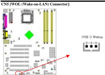
Enable the Power ON by Ring selection in BIOS's Power Management Menu to use this function. This header is used to connect an add-in NIC (Network Interface Card) which gives WOL capability to the motherboard.
