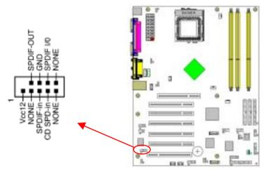
This connector must be connected to a SPDIF bracket.
