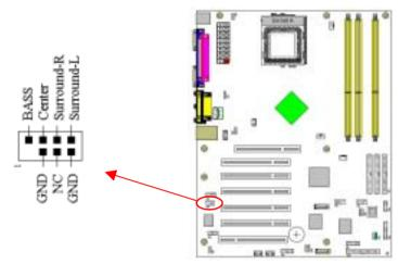
This connector must be connected to a 6-channel bracket.
