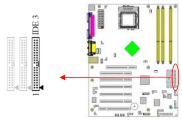
This connector is used for connecting IDE HDD, which builds IDE RAID. Using IDE RAID, the IDE HDD needs to be set to Master, not Slave; otherwise, the HDD can not be detected. For 7NJS, <u>one/two Serial ATA(s) and</u> <u>one IDE RAID</u> or <u>two Serial ATAs</u> need to be used at the same time. Otherwise, single HDD, which is plugged in IDE RAID or Serial ATA can not be become RAID function.
