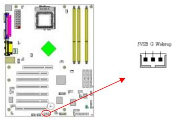
Enable the Power ON by Ring selection in BIOS's Power Management Menu to use this function. This header is used to connect an add-in modem card which gives WOM capability to the motherboard.
