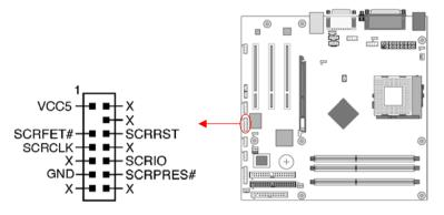
This connector must be connected to a Smart card reader, which allows you to transfer data through Smart Cards and Smart Card user interface software.
