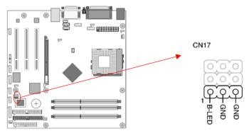
These features work entirely the same as the power indicator LED, both shows the system's power status. The only difference is that this one is blue while the other is red LED.
