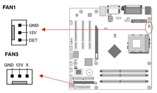
The board's management extension hardware is able to detect the CPU fan speed in rpm (revolutions per minute). The wiring and plug may vary depending on the manufacturer. On standard fans, the red is positive (+12V), the black is ground, and the yellow wire is the rotation signal.
