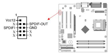
This connector must be connected to a **SPDIF bracket**. This will allow you to use the SPDIF option.
