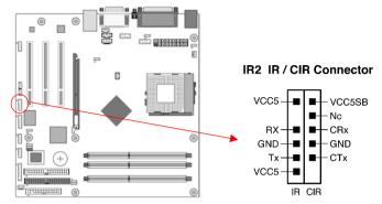
Select a UART Mode in BIOS's Integrated Peripherals menu the UART port to support IR function. (See section 3 Super I/O Device of Integrated Peripherals)
