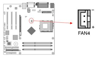
The north bridge-cooling fan. The wiring and plug may vary depending on the manufacturer. On standard fans, the red is positive (+12V), the black is ground.
