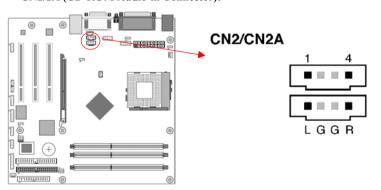
Use the audio cable enclosed with your CD-ROM disk drive to connect the CD-ROM drive onto your motherboard. This will enable your CD-ROM's audio function.
