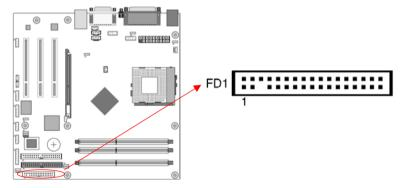
This motherboard provides a standard floppy disk drive connector that supports 360K, 720K, 1.2M, 1.44M and 2.88M floppy disk types. This connector is used to connect 34 pins of Floppy drive cable.
