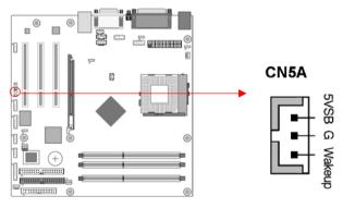
The Wake Up On Modem selection in BIOS's Power Management Setup Menu must be enabled to use this function. This header is used to connect an add-in modem card, which gives WOM capability to the motherboard.
