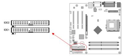
This connector is used for connecting 40 pins of ATAPI devices.
