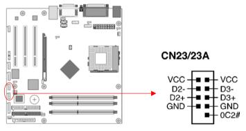
If you want to use a USB Keyboard, you must enable the USB keyboard support function in BIOS's Integrated Peripherals menu (See Section 3). This board contains a USB Host controller and includes a root hub connector for optional USB Adaptor (USB 2/3 and 4/5).
