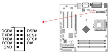
This is an addition 9-pin connector is for a serial port ribbon cable. This will allow you to enable an additional COM Port.
