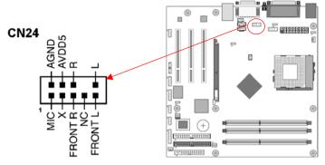
This connector give you the option of a front panel audio jack cable ext. to be plug into a special custom designed system case. Simply remove the two jumper caps at pin [5-6] and [9-10] then plug it into the (optional) cable ext. connector. Pin [5-6] and [9-10] are shorted (default) to enable the back panel audio function.
