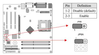
A USB keyboard hot key or a USB mouse click can turn on this motherboard. To use this function, select [Enable] at the USB Resume from S3 under Wake Up Events in the BIOS's Power Management setup screen. You must also set this jumper's cap to pins [2-3] to use this function.
