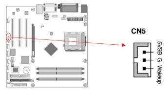
Enable the Wake Up On LAN selection in BIOS's Power Management Setup Menu to use this function. The capability to remotely manage PCs on a network is a significant factor in reducing administrative and ownership costs. Magic Packet technology is designed to give WOL capability to LAN controller. This header is used to connect an add-in NIC (Network Interface Card) that gives WOL capability to the motherboard.
