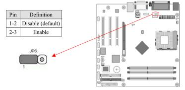
A USB keyboard hot key or a USB mouse click can turn on this motherboard. To use this function, select [Enable] at the USB Resume from S3 under Wake Up Events in the BIOS's Power Management setup screen. You must also set this jumper's cap to pins [2-3] to use this function.
