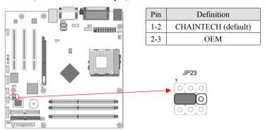
This motherboard provides a Green LED flash Jumper. This cap is to setup Green LED flash mode. The default value is [1-2], which is manufacture defined. For user defend or OEM please set the jumper cap at [2-3].
