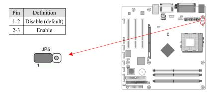
This board can be turned on by the PS / 2 keyboard (hot key). To use this function, select a hot key of your choice at the Power On Function option under Wake Up Events in the BIOS's Power Management setup screen. You must also set this jumper's cap to pins 2-3 to use this function.
