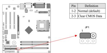
There is a CMOS RAM on board that has a power supply from external battery to keep the data and system configuration. To clear the contents of the CMOS, please follow the steps below.
