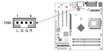
These connectors are for CD-Rom devices audio. It is for Auxiliary Audio-in Device, which will input the sounds sources into the motherboard.
