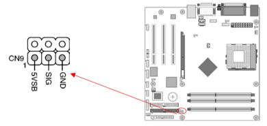
This connector is for a chassis open alarm; it provides a buzzer sound when an attempt to open the chassis occurs.
