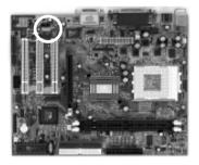
2Use the auxiliary audio cable enclosed with your CD-ROM disk drive to connect the CD-ROM to your mainboard. This will enable your CD-ROM's audio function.
