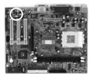
This connector must be connected to the cable from the voice modem card to support modem audio signals.
