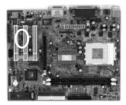
Select an IR mode at the UART 2 Mode in BIOS Integrated Peripherals menu to enable the IR functions on this mainboard. (See Section 3-4)
