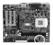
This switch allows you to select between 100MHz FSB or 133MHz FSB frequency speed. You must set the jumper's cap to pins 1-2 for 100MHz or set the jumper's cap to pins 2-3 for 133MHz FSB.
