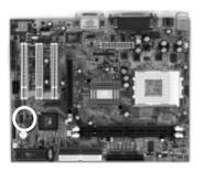
This board contains a connector for an optional USB Adaptor (USB2/3). Four USB peripherals or hub devices are able to be connected.
