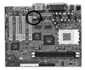
Use the auxiliary audio cable enclosed with your CD-ROM disk drive to connect the CD-ROM to your mainboard. This will enable your CD-ROM's audio function.
