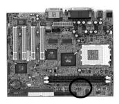
This switch allows you to select between 100MHz FSB or 133MHz FSB frequency speed.
