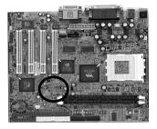
This connector is to be connected to an optional LCD/TV-out adapter card.
