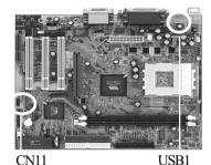
If you want to use a USB keyboard, you must enable the USB keyboard support function in BIOS's Integrated Peripherals menu (See Section 3-4).
