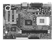
The S/PDIF-Out connector supports the digital audio. This connector must be connected to the cable from an external device. (Ex. 2-channel decoded AC-3 from DVD decoders)
