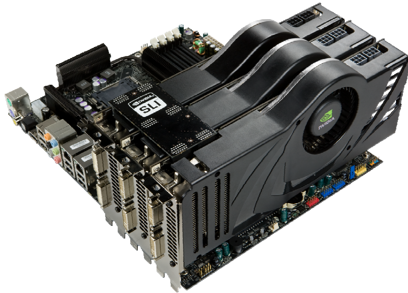
Figure 17. 3-Way SLI Using GeForce 8800 Ultra
