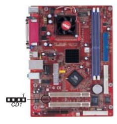
When you first start up your system, the BIOS should automatically detect your CD-ROM/DVD drive. If it doesn't, enter the Setup Utility and configure the CD-ROM/DVD drive that you have installed. On the motherboard, locate the 4-pin header CD1.
