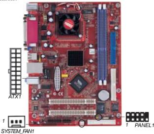
Connect the power connector from the power supply to the **ATX1** connector on the motherboard.
