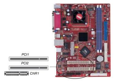
Follow the steps below to install a CNR/PCI expansion card.
