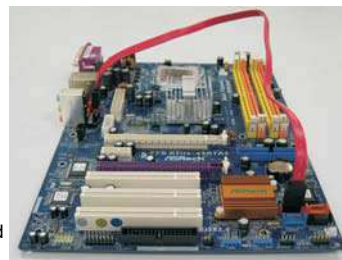
Connect the SATA data cable to the red eSATAII connector (eSATAII_BOTTOM)
