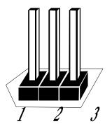
**CPU Fan** A three-pin berg labeled FAN attaches to the CPU fan. The FAN connector is next to the CPU socket.
