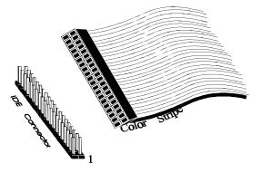
IDE1 is a 40-pin dual-inline berg that connects an IDE drive to the primary onboard IDE connector. This motherboard supports IDE Modes 0, 1, 2, 3, and 4, IDE prefetch, LBA (Logical Block Address) mode, high capacity drives (over 528 MB), 32-bit data transfer, and fast IDE transfer. These IDE features are configured in Peripheral Setup in the WINBIOS Setup utility. Disable the onboard IDE interface in Peripheral Setup to use an ISA ESDI, RLL, MFM, or SCSI hard disk drive controller.
