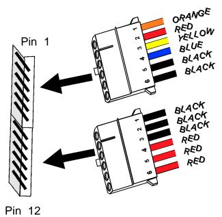
**Connector Keys** The keys on the connector must be cut to fit on some power supplies, as shown below.
