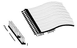
The motherboard supports up to two 720 KB, 1.44 MB, or 2.88 MB 3<sup>1</sup>/<sub>2</sub>" drives and 360 KB and 1.2 MB 5<sup>1</sup>/<sub>4</sub>" drives. The connecting cable is a 34-pin ribbon connector with two 34-pin edge connectors for attaching the floppy disk drives. There is a small twist in the cable between the floppy connectors. The last (end) connector should be connected to floppy drive A:.
