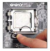
11. Press the four hooks down to fasten the cooler. Then rotate the locking switch (refer to the correct direction marked on it) to lock the hooks.
