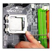
Press down the load lever lightly onto the load plate, and then secure the lever with the hook under retention tab.
