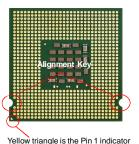
The surface of LGA 775 CPU. Remember to apply some thermal paste on it for better heat dispersion.
