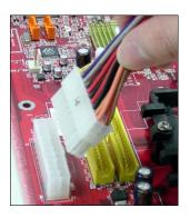
Figure 2: Unplug the power connector
