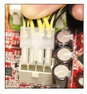
Figure 3: Unplug the power connectors
