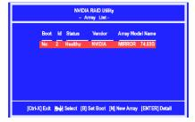
Use the arrow keys to select the array that you want to set up, then press Enter. The Array Detail window appears.
