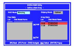
It shows that two disks have been assigned as RAID1 array disks in the figure above.
