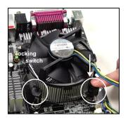
Align the holes on the mainboard with the heatsink. Push down the cooler until its four clips get wedged into the holes of the mainboard.
