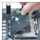
Yellow triangle is the Pin 1 indicator
