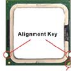
Yellow triangle is the Pin 1 indicator
