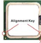
Yellow triangle is the Pin 1 indicator
