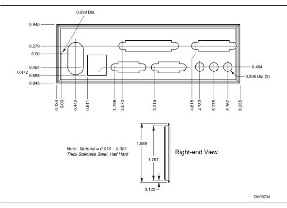
Figure 9. Back Panel I/O Shield Dimensions (ATX Chassis-Independent)
