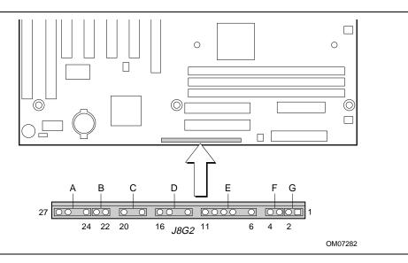
Figure 5. Front Panel I/O Connectors
