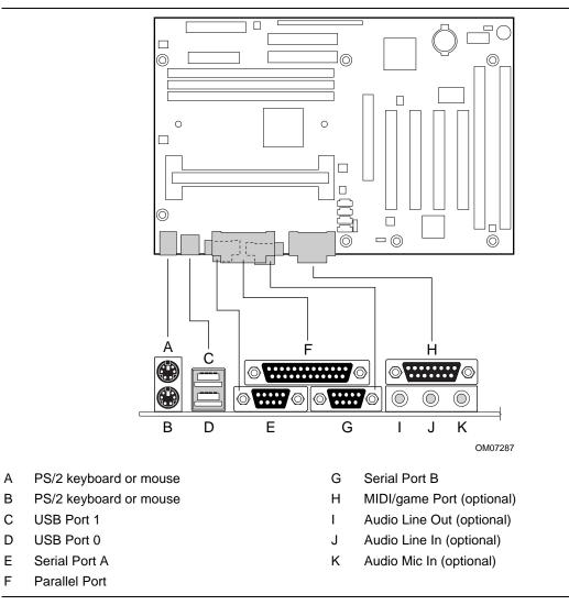
Figure 3. Back Panel I/O Connectors
