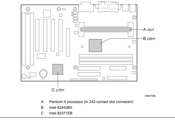
Figure 10 shows motherboard components that may be sensitive to thermal changes.
