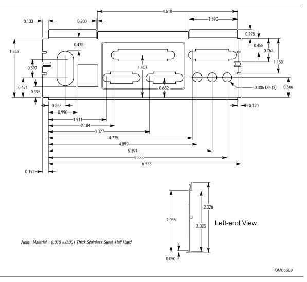
Figure 8. Back Panel I/O Shield Dimensions (ATX Chassis-Dependent)
