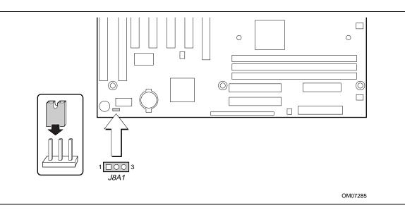
Figure 6. Location of the Configuration Jumper Block
