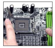
After confirming the CPU direction for correct mating, put down the CPU in the socket housing frame. Be sure to grasp on the edge of the CPU base. Note that the alignment keys are matched.
