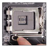
2. Remove the cap from lever hinge side (as the arrow shows).
