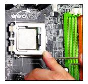
9. Press down the load lever lightly onto the load plate, and then secure the lever with the hook under retention tab.
