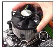
12. Turn over the mainboard to confirm that the clip-ends are correctly inserted.
