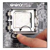
Press the four hooks down to fasten the cooler. Then rotate the locking switch (refer to the correct direction marked on it) to lock the hooks.
