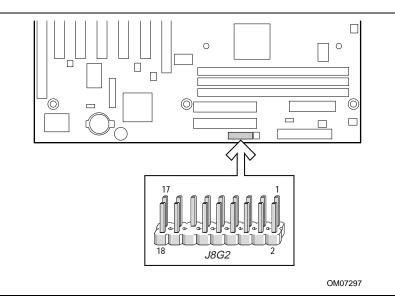
Figure 6. Double Row Front Panel I/O Connector
