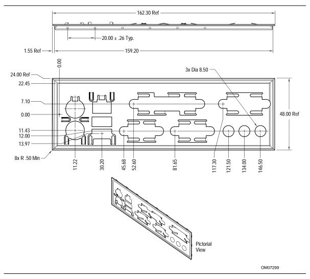
Figure 9. Back Panel I/O Shield Dimensions (ATX Chassis-Dependent)
