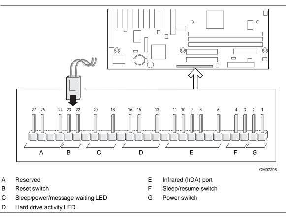
Figure 5. Single Row Front Panel I/O Connector
