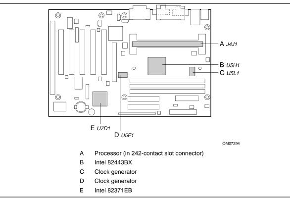
Figure 10. Thermally-Sensitive Components
