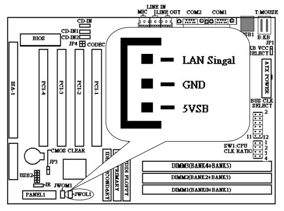
For supporting this feature, the system must have a ATX Power Supply), that must provide at least 800mA driving ability on the "5V standby" voltage
