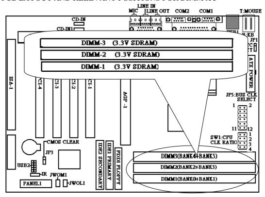
(2) The Supports Different Type Of Settings For The System Memory . There Is No Jumper Nor Connect Needed For Memory Configuration . Following Figures Provides All Possible Memory Combinations .
