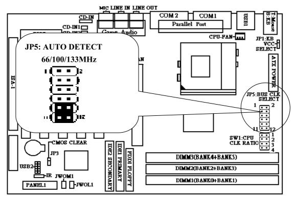
The M/B Design Auto-Detect CPU BUS CLK 66 & 100 & 133 MHZ Frequency \* No Jumper Needed For Setting .
