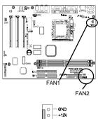
These added connectors allow the fan to draw their power from the mainboard instead of the disk drive connector.
