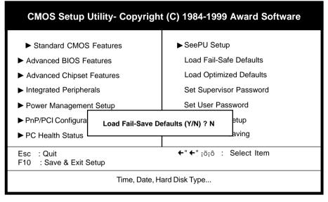
Figure 3-10 Load Fail-Safe Defaults Screen
