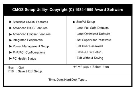
Figure 3-1 Setup Program Initial Screen
