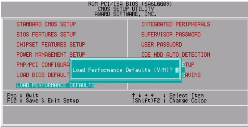
Figure 4.8: Load Performance Defaults
