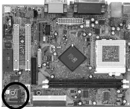
If you enable the IR/CIR Address Select in BIOS's Integrated Peripherals menu the IR/CIR port will let you select the IRQ and IR/CIR Mode to support IR/CIR functions. Connect this connector to the IR/CIR devices to enable this function.
