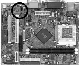
Use the cable enclosed with your CD-ROM disk drive to connect the CD-ROM to your mainboard. This will enable your CD-ROM's audio function.
