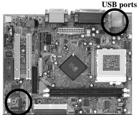
If you want to use a USB keyboard, you must enable the USB keyboard support function in BIOS's Integrated Peripherals menu (See Section 3-4). USB is an open industry standard, providing a simple and inexpensive way to connect up to 125 devices to a single computer port. Keyboards, mice, tablets, digitizers, scanners, bar-code readers, modems, printers and many more can all be used at the same time.
