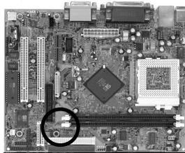
The I<sup>2</sup>S Connector supports the MPEG sound decoder. This connector must be connected to the cable from the MPEG card.
