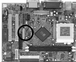
This connector is to be connected to an optional TV/LCD/2nd CRT Output adapter card.
