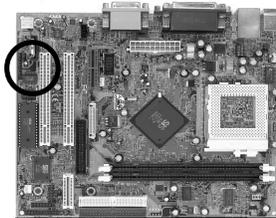
This optional connector must be connected to a speaker out and Mic-in jack adaptor.
