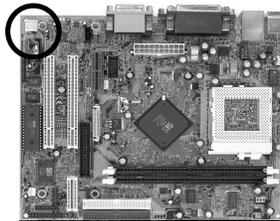
Use the mono audio cable enclosed with your CD-ROM disk drive to connect the CD-ROM to your mainboard. This will enable mono audio in/out function.
