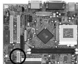
This connector is to be connected to a PCI riser card (optional) for additional PCI slots support.
