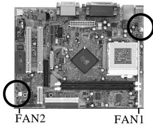
These added connectors allow the fan to draw their power from the mainboard instead of the disk drive connector. The board's management extension hardware is able to detect the CPU and system fan speed in rpm (revolutions per minute). These connectors supports 3-pin cooling fans with minimum of 3500RPM. The wiring and plug may vary depending on the manufacturer. On standard fans, the red is positive (+12V), the black
