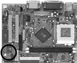
The S/PDIFconnector supports the digital audio. This connector must be connected to the cable from an external device. (Ex. 2-channel decoded AC-3 from DVD decoders)
