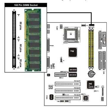
The Dual Inline Memory Module (DIMM) memory module must be 3.3v Extended Data Output (EDO) DRAM or SDRAM. You can identify the type of DIMM module by the illustration below:
