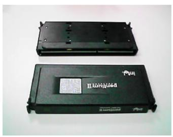
Figure 2:OEM Pentium® II Processor
