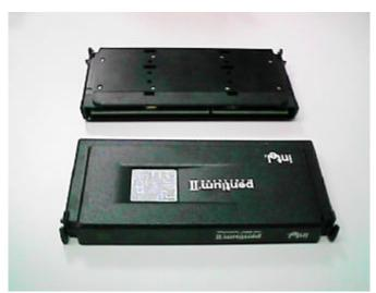
Figure 2:OEM Pentium® II Processor
