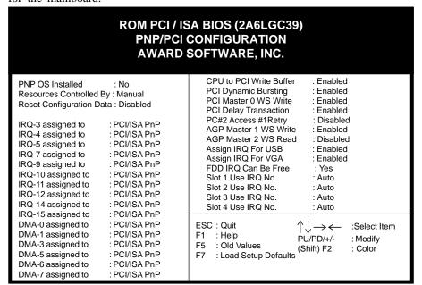
Figure 3-6 PCI & ONBOARD I/O Setup Screen
