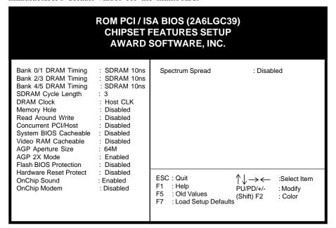
Figure 3-4 Chipset Features Setup Screen
