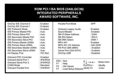
Figure 3-9 Integrated Peripherals Setup Screen
