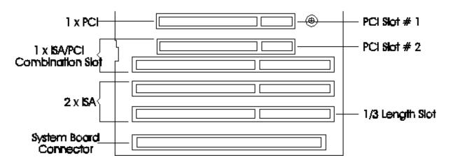
The right-hand side, as viewed from the front of the PC, has the new PCI slot that accommodates the Enhanced Ethernet 10 BaseT Network board.
