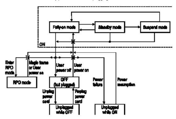
The following diagram gives a more accurate, more detailed account of the valid state changes. It highlights two limitations of the RPO system: power-off before the operating system boot procedure has initialized the RPO function, or a power failure whilst the system in RPO mode, will each de-activate the RPO function.
