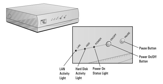
Power On/Off Button Press this button to turn the power on or off to your PC.
