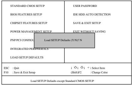
Figure 4.7: Load Setup Defaults
