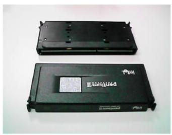
Figure 2:OEM Pentium® II Processor
