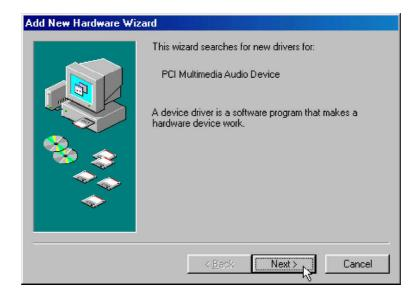
2. As Windows95/98 starts up, it will automatically detect the audio controller and start the driver installation. Winows95/98 will detect the audio controller as " PCI Multimedia Audio Device" The Wizard will guide you to begins the driver installation.
