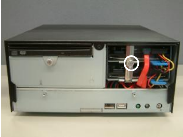
a. Loosen the thumb screw (1).
