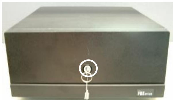
a. Use the key to unlock the front cover
