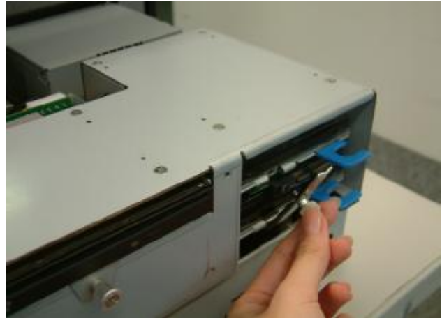
b. Loosen the locking bar (1).
