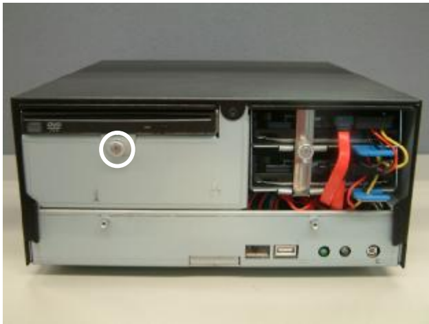
a. Loosen the thumb screw (1)
