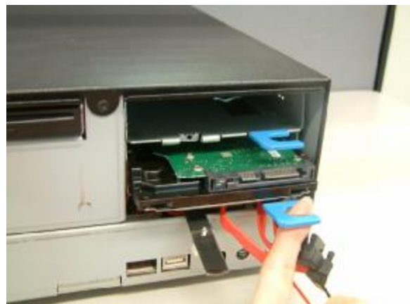
f. Repeat the step d. and e. to remove the other HDD.
