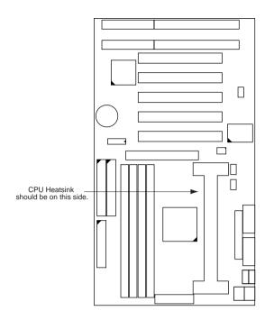
The retention clip should be inserted so that the small rectangle window is more toward to the right hand side of the board.
