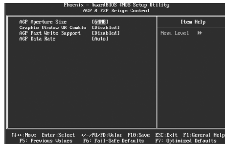
AGP & P2P Bridge Control Menu
