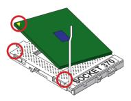
Take notice of the red circles as shown below. While inserting the CPU into the socket, you can find out there is a definite pin orientation for CPU and socket.
