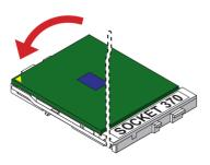
Make sure that the CPU is placed into the socket tightly.
