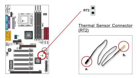
We provide a thermal cable in the mainboard package. This thermal cable is to monitor device which will generate a lot of heat, such as HDD, graphics card etc.. Please connect one end of the thermal cable (A) to mainboard RT2 header, and tape the other end of thermal cable (B) on to the device which you want to monitor. After you finish the thermal cable installation, you will see the detected temperature in BIOS setup or Hardware monitor utility.
