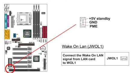
This connector connects to a LAN card with a Wake On LAN output. The connector powers up the system when a wake-up packet or signal is received through the LAN card.
