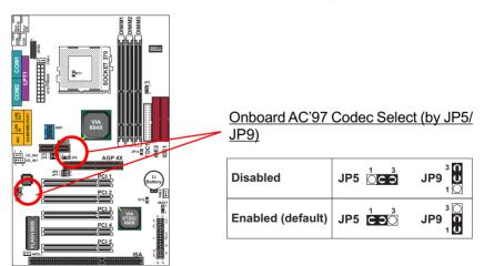
If there is Audio/Modem AMR card on the motherboard using primary channel, the on-board AC'97 codec must be disabled.
