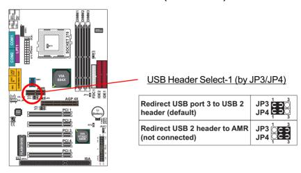
USB2 Header Select1 by JP3/4 is for future use when there is a need to connect USB2 Header to AMR. Currently, USB2 to AMR is not connected. Please keep use default setting to enable USB2 Header.
