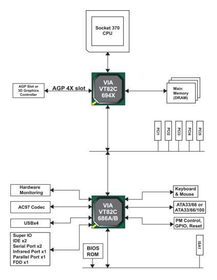
Figure 1-11. VIA VT694X System Block Diagram Using the VT82C686A or VT82C686B South Bridge
