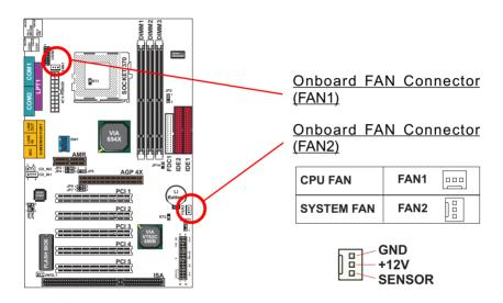
These connectors support CPU/System cooling fan with +12V. When connecting wire to FAN connectors, users should pay attention that the red wire is for the positive current and should be connected to pin +12V, and the black wire is Ground and should be connected to pin GND. If your mainboard has Hardware Monitor chipset on-board, you must use a specially designed fan with speed sensor to take advantage of this function.
