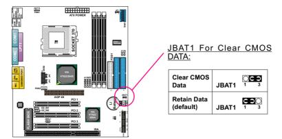
NOTE: You can clear CMOS by 2-3 pin when the system is POWER OFF. Then, return to 1-2 pin position (default). It may damage the mainboard if clearing the CMOS with POWER ON. Unplugging the power cord from power supply before clearing CMOS will be a safest bet for user.
