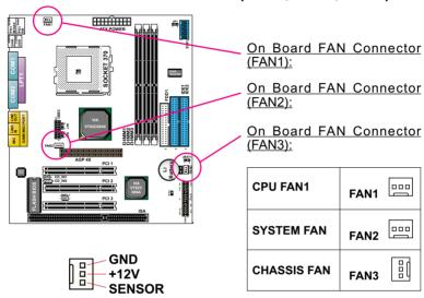
These fan connectors support CPU/System chassis cooling fan with +12V. When connecting wire to FAN connectors, users should pay attention that the red wire is for the positive current and should be connected to pin +12V, and the black wire is Ground and should be connected to pin GND. If your mainboard has Hardware Monitor chipset on-board, you must use a specially designed fan with speed sensor to take advantage of this function.
