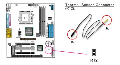
We provide a thermal cable in the mainboard package. This thermal cable is to monitor device which will generates a lot of heat, such as HDD, Graphics card etc. Please connect one end of the thermal cable (A) to mainboard RT2 header, and tape another end of thermal cable (B) on to the device which you want to monitor. After you have finish the thermal cable installation, you will see the detected temperature in BIOS setup or Hardware monitor utility.
