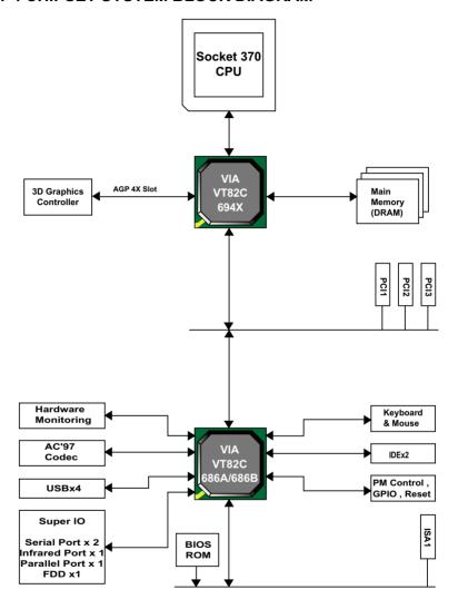
Diagram of VIA VT86C694X System Block with VT82C686A or VT82C686B South Bridge
