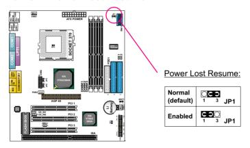
NOTE: This jumper allows user to use the switch of ATX power supply to control ON/OFF switch directly instead of using the power switch on the mainboard.
