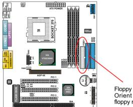
Floppy Disk Drive Connector: Orient the red line on the floppy ribbon cable to Pin1.
