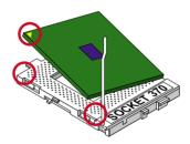
Make sure that the CPU is placed into the socket tightly. Then lower down the lever to complete the CPU installation.
