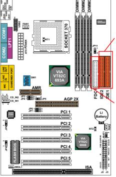
Hard Disk Drive Connector: Orient the red markings on the IDE ribbon cable to Pin1.
