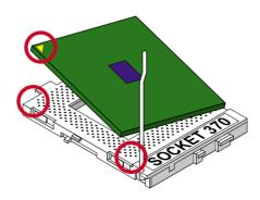
3. Make sure that the CPU positions in the socket tightly, and then put the lever down to complete the CPU installation.
