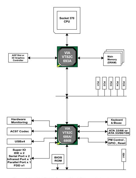
Figure 1-11. VIA VT693A System Block Diagram Using the VT82C686A or VT82C686B South Bridge
