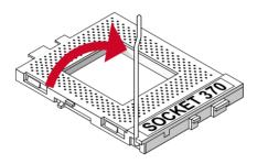
Take note of the red circle as below picture. When insert the CPU into socket, you can find out there is a definite pin orientation for CPU and socket.
