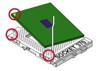
Take notice of the red circles as shown below. While inserting the CPU into the socket, you can find out there is a definite pin orientation for CPU and socket.
