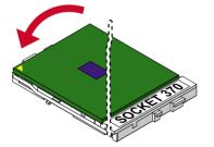
Make sure that the CPU is placed into the socket tightly. Then lower down the lever to complete the CPU installation.
