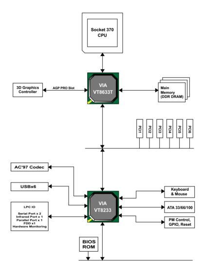
Diagram of VIA VT8633T System Block Using the VT8233 South Bridge
