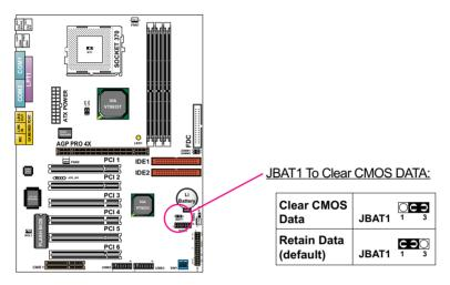
**NOTE:** You can clear CMOS by setting Pin 2-3 closed when the system is POWER OFF. Then, return to Pin1-2 position (default). You may damage the mainboard if clearing the CMOS with POWER ON. Unplugging the power cord from power supply before clearing CMOS will be the safest bet for user.
