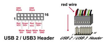
• When plugging the USB cable into USB2/USB3 HEADER, users must make sure the red wire is connected to the first pin.
