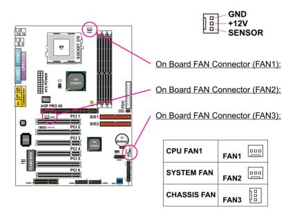
These connectors support CPU/System/chassis cooling fan with +12V. When connecting wire to FAN connectors, users should pay attention that the red wire is for the positive and should be connected to pin +12V, and the black wire is Ground and should be connected to pin GND. If your mainboard has Hardware Monitor chipset on-board, you must use a specially designed fan with speed sensor to take advantage of this function.
