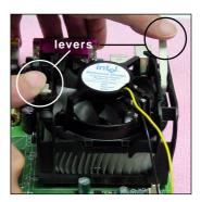
Connect the fan power cable from the mounted fan to the 3-pin fan power connector on the board.
