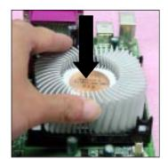
Mount the fan on top of the heatsink. Press down the fan until its four clips get wedged in the holes of the retention mechanism.
