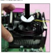
**4.** Press the two levers down to fasten the fan. Each lever can be pressed down in only ONE direction.
