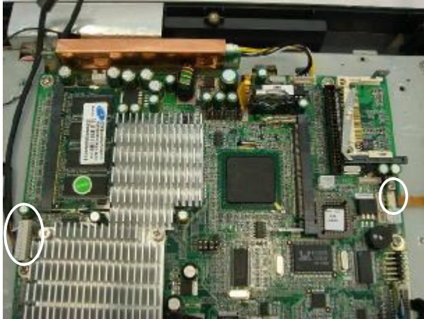
a. Disconnect the cables (2): card reader cable and touch cable.
