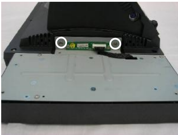
e. Tighten the screws (2) to secure the keypad.
