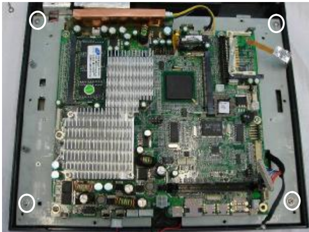
c. Remove the screws (4) to separate the LCD panel and touch screen.
