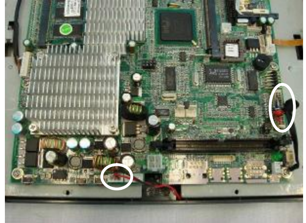
b. Disconnect the cables (2): power/LAN LED cable and LCD Interface cable.
