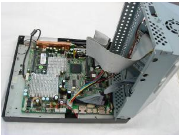
i. Lift the base chassis to disengage it from the LCD chassis and place it next to the LCD chassis, taking care not to stretch the cables which are still connected.
