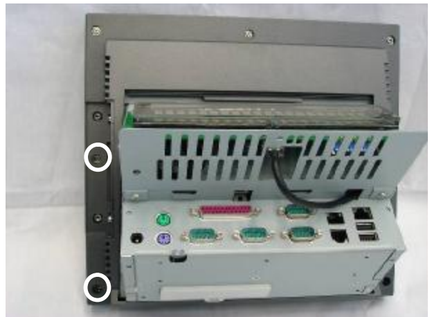
d. Remove the screws (2) to lift the LCD back cover up.
