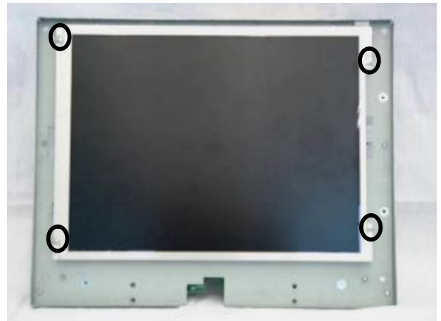
d. Remove the screws (4) to replace the LCD panel.
