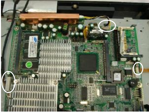
a. Disconnect the cables (3): card reader cable, inverter cable and touch cable.
