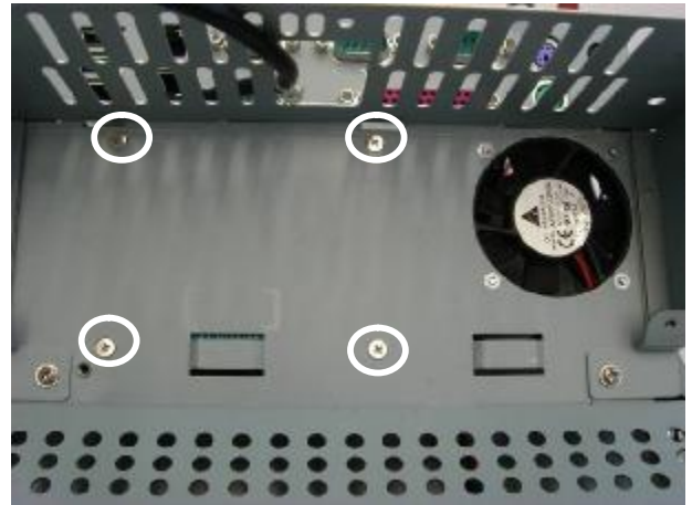
f. Remove the screws (4) to replace the HDD.
