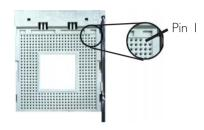
4. Insert the CPU into the socket until it is seated in place. The CPU will fit in only one orientation and can easily be inserted without exerting any force.
