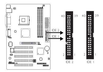
The system board is equipped with two shrouded PCI IDE headers that will interface four Enhanced IDE (Integrated Drive Electronics) disk drives. To prevent improper IDE cable installation, each shrouded PCI IDE header has a keying mechanism. The 40-pin connector on the IDE cable can be placed into the header only if pin I of the connector is aligned with pin I of the header.
