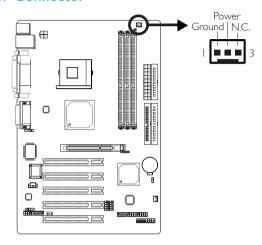
The CPU must be kept cool by using a fan with heatsink. Connect the CPU fan to the 3-pin fan connector at location JI5 of the system board.
