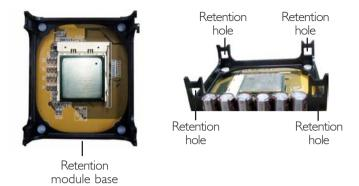
2. Position the fan / heat sink and retention mechanism assembly on the CPU, then align and snap the retention legs' hooks to the retention holes at the 4 corners of the retention module base.
