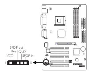
The system board is equipped with a S/PDIF connector. One cardedge bracket, mounted with S/PDIF ports, will be provided as an option. Install the card-edge bracket to the system chassis then connect the audio cable connector to J4. Make sure pin I of the audio cable connector is aligned with pin I of J4.
