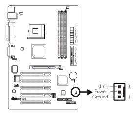
The chassis fan connector (J21) is used to connect a cooling fan. The cooling fan will provide adequate airflow throughout the chassis to prevent overheating the CPU and system board components.
