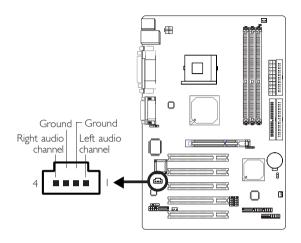
The CD-in (J5) connector is used to receive audio from a CD-ROM drive. TV tuner or MPEG card.
