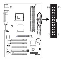
The system board is equipped with a shrouded floppy disk drive connector that supports two standard floppy disk drives. To prevent improper floppy cable installation, the shrouded floppy disk header has a keying mechanism. The 34-pin connector on the floppy cable can be placed into the header only if pin I of the connector is aligned with pin I of the header.
