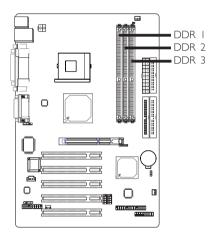
The system board supports DDR SDRAM DIMM. Double Data Rate SDRAM (DDR SDRAM) is a type of SDRAM that doubles the data rate through reading and writing at both the rising and falling edge of each clock. This effectively doubles the speed of operation therefore doubling the speed of data transfer.
