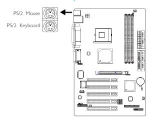
The system board is equipped with an onboard PS/2 mouse (Green) and PS/2 keyboard (Purple) ports - both at location CNI of the system board. The PS/2 mouse port uses IRQ12. If a mouse is not connected to this port, the system will reserve IRQ12 for other expansion cards.
