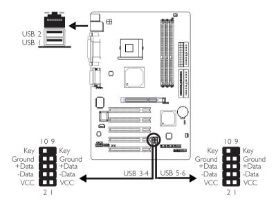
Two onboard USB 2.0/1.1 ports (Black) are at locations CN7 of the system board.
