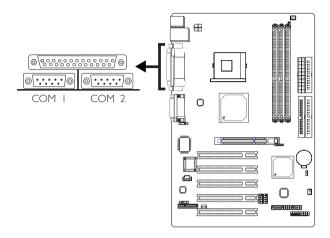
The system board is equipped with two onboard serial ports (COM I: CN6 and COM 2: CN5) - both in Teal/Turquoise color.
