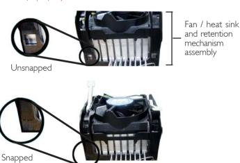
3. The retention levers at this time remains unlocked as shown in the illustration below.
