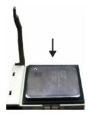
Once the CPU is in place, push down the lever to lock the socket. The lever should click on the side tab to indicate that the CPU is completely secured in the socket.
