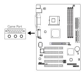
The Game/MIDI port is identical to that of a standard PC game adapter or game I/O port. Connect an analog joystick to the I5-pin D-sub connector (Gold) at location CN8 of the system board. This port works well with any application that is compatible with the standard PC joystick.
