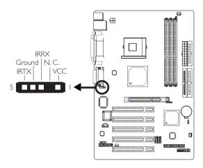
Connect your IrDA cable to connector |2 on the system board.
