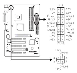
We recommend that you use a power supply that complies with the ATX12V Power Supply Design Guide Version I.I. An ATX12V power supply has a standard 20-pin ATX main power connector and a 4-pin +12V power connector that must be inserted onto CNII and CNIO connectors respectively.
