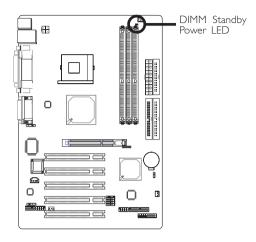
The DIMM Standby Power LED will turn red when the system's power is on or when it is in the Suspend state (Power On Suspend or Suspend to RAM). It will not light when the system is in the Soft-Off state.
