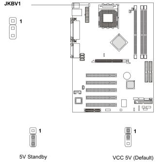
5V Standby Enable Keyboard Power On function
