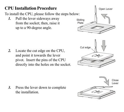
**Note:** The CPU is designed with the "corner pin" on the two of the four corners; thus, it should only fit in one correctly orientation as installing. In addition, with the weight of the heatsink and cooling fan attached, you can insert the CPU into the socket easily. **DO NOT** press the CPU down by force when installing in wrong orientation, this would bend and damage
