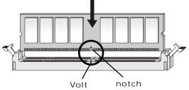
**3.** The plastic clip at each side of the DIMM slot will automatically close.
